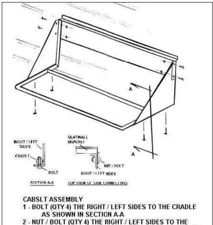
2 - NUT / BOLT (QTY 4) THE RIGHT / LEFT SIDES TO THE SLATWALL BRACKET AS SHOWN IN THE "TOP VIEW"
