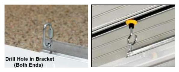
Step #2: Attach the S hook directly to a pair of ring hanger hooks in a PowerTrak rail or to a ring hook screwed into a ceiling joist. For higher ceilings, use a light duty chain to drop the fixture to the height you desire.
